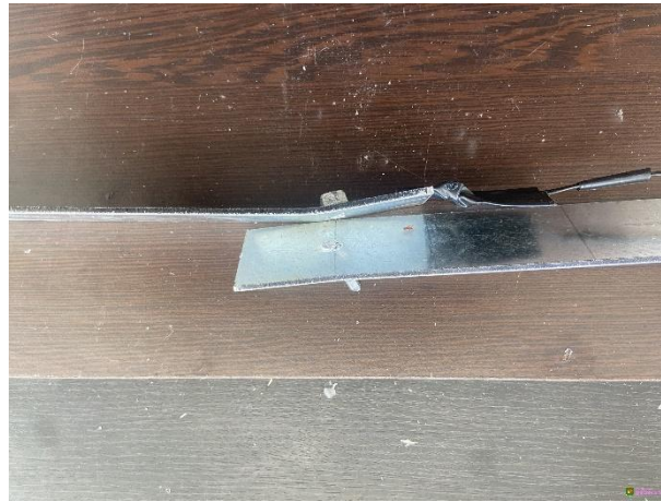
(b) S type failure
