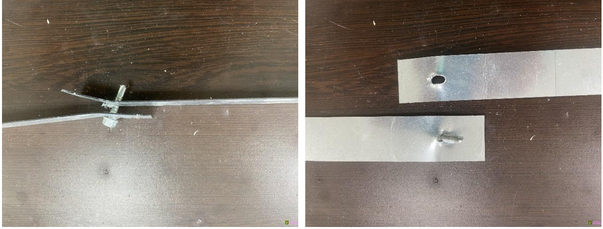
(a) T-B type failure
