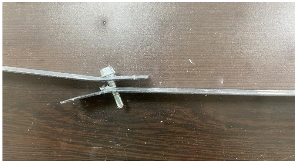
(a) T-B type failure
