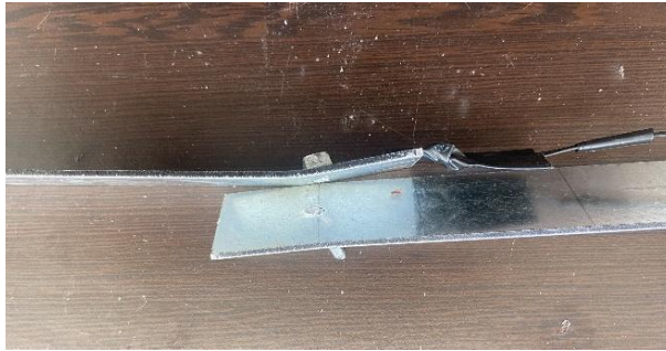
(b) S type failure
