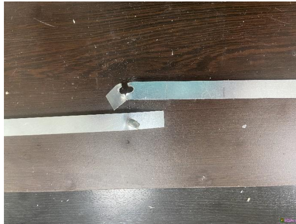
(c) NS type failure
