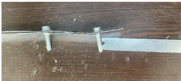
(b) S type failure
