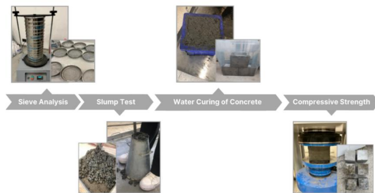
Figure 3. Schematic representation of the stepwise test procedure of CC and 0.5CF specimens.
