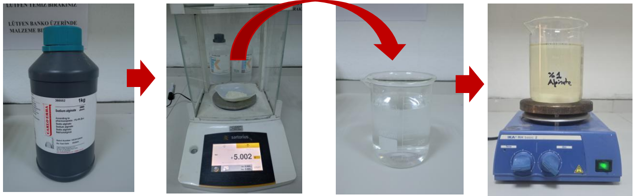
Figure 4. Images of the preparation of alginate solutions.
