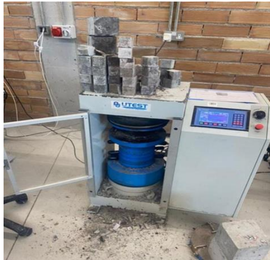
Figure 8. Compressive strength testing.
