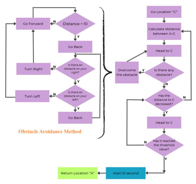
Figure 5. Flow Diagram of the Direction Detection Algorithm
