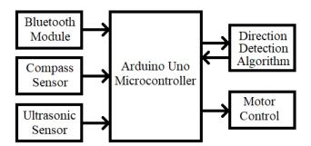
Figure 1. Working Principle of the Cargo Carrier Robot
