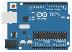
Figure 2. Arduino Uno R3 Microcontroller [16]
