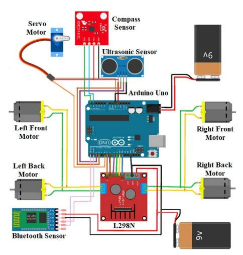
Figure 7. Block Diagram of Cargo Carrier Robot
