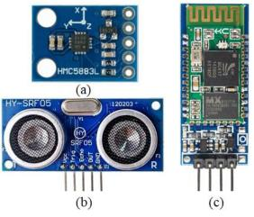
Figure 3. Cargo Carrier Robot Sensing Unit
