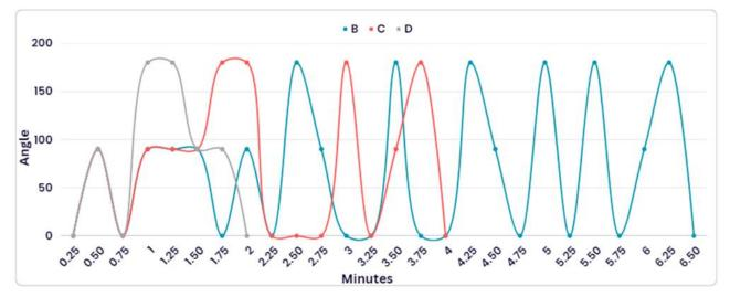
Figure 9. Angle-Time Graph of the Servo Motor
