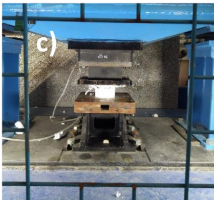
Figure 3. Drop weight test set-up a) schematic view (1: hammer head 2: load cell 3: displacement sensor 4: support plate 5: test specimen) b) detailed view of the test specimen #1 on the support plate c) overall view.
