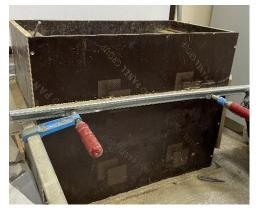
Figure 2. Displacement-controlled pile model unit
