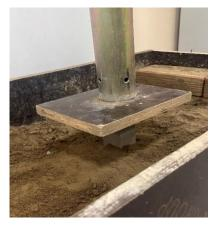
Figure 4. Displacement pile application process
