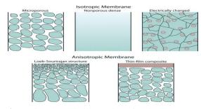
Figure 1. Schematic illustration of various classes of membranes.
