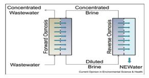
**Figure 4.** Integrating FO and RO methods for energy optimization. The RO brine would play the role of the draw solution in that NEWater production scheme.
