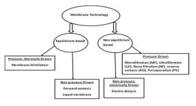
Figure 3. Schematic representation of some membrane processes
